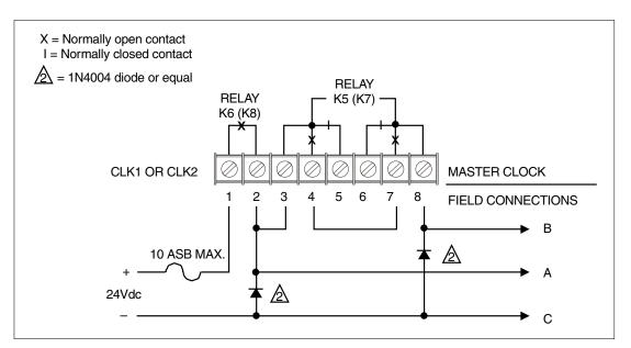
Figure B-2 Three-Wire Minute Impulse (59th Minute)
